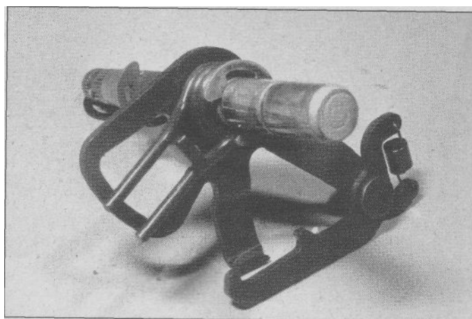
18.7b Remove the C-clip at each end of the shaft and slide the parts off for inspection
