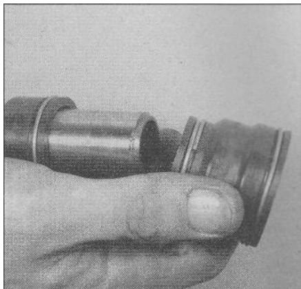
9.8a Slide the boot off the coupling gear
