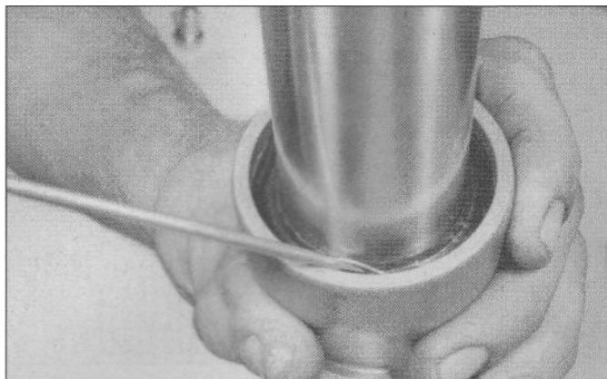
5.5 Pry out the retaining ring
