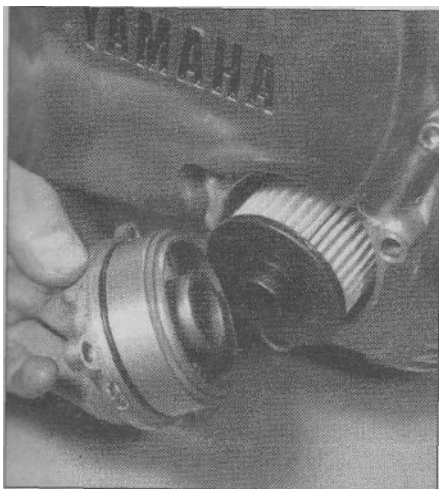
13.6a ... and remove the cover together with its two O-rings
