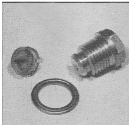
7.27 Check the needle valve seat for wear; check the filter cap for clogging or tears; replace the sealing washer with a new one
