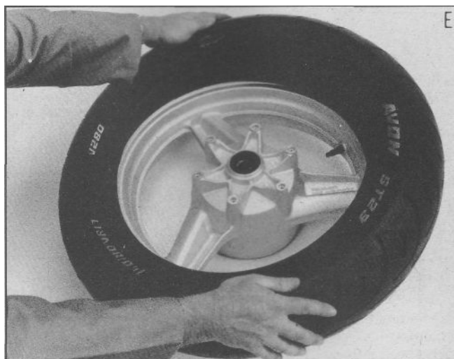
Work first bead over the rim flange.
