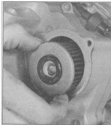
13.6b Pull the filter element out of the engine
