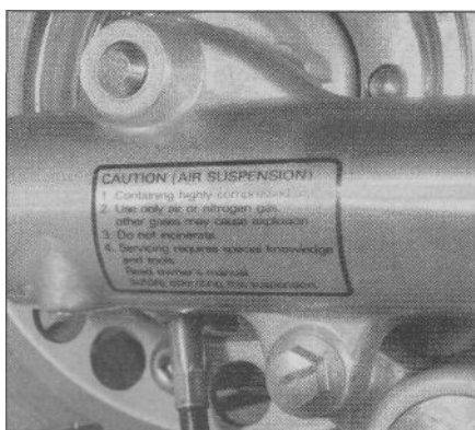
2.3b ... special precautions for air-adjustable front forks ...
