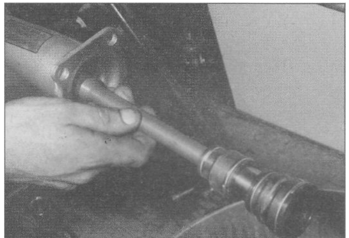
9.7 Pull the driveshaft backward and take it out of the swingarm
