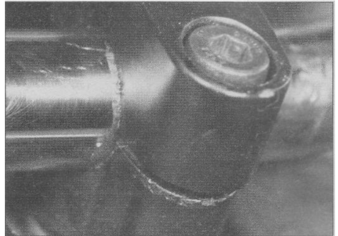
2.7b Align the dot on the handlebar with the gap in the bracket; the gaps at front and back of the bracket must be even
