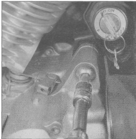
5.25c ... (there's an upper rear mounting bolt on each side of the engine)
