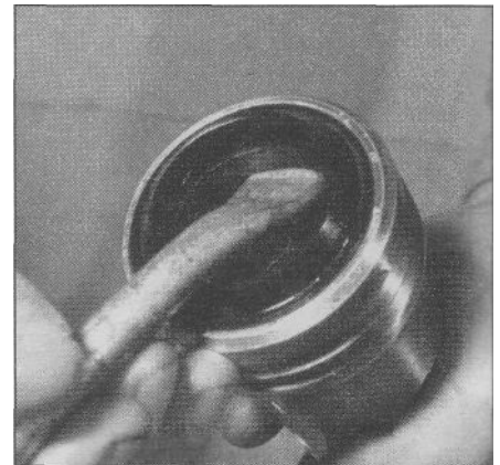
8.8 Pry the oil seal out of the lower fork tube
