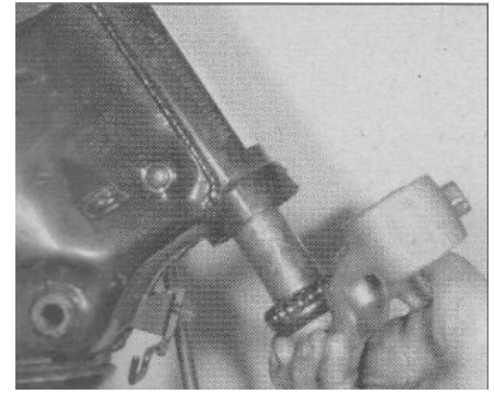
6.17 Slip the steering stem into the steering head, taking care not to dislodge the steel balls
