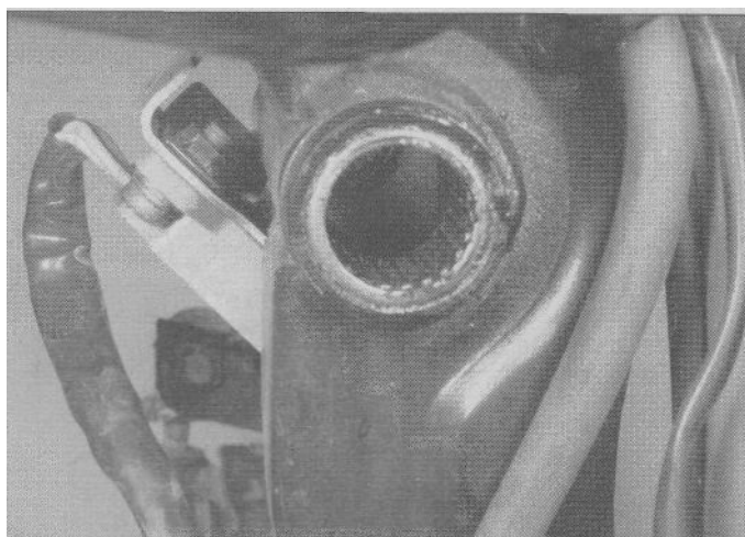
11.4 The bearings may require a blind hole puller for removal
