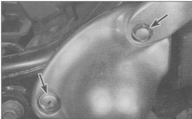
7.2 Remove the shock absorber cover fasteners (arrows); on some models one of the fasteners also secures the backrest
