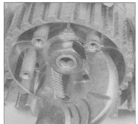
16.31 Once the nut is tightened to the specified torque, bend the lockwasher against the nut
