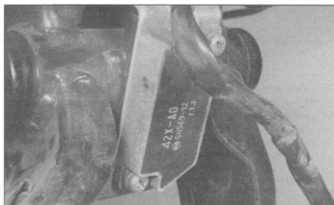
28.13 The regulator/rectifier on early models is mounted on the lower rear portion of the frame
