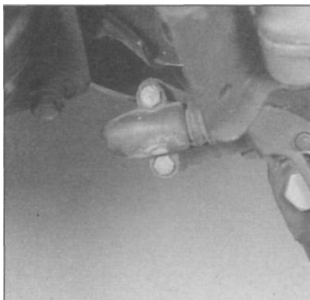
19.5 Sidestand switch mounting screws
