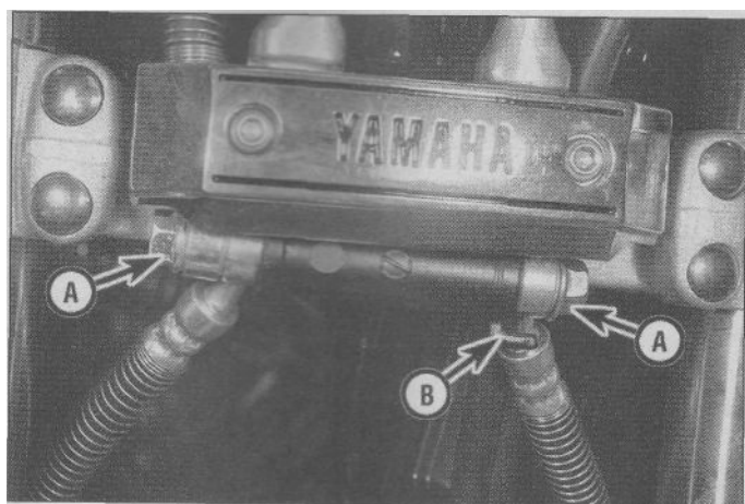
7.2 Remove the union bolts (A); note the position of the banjo fitting neck next to the cast lug (B)
