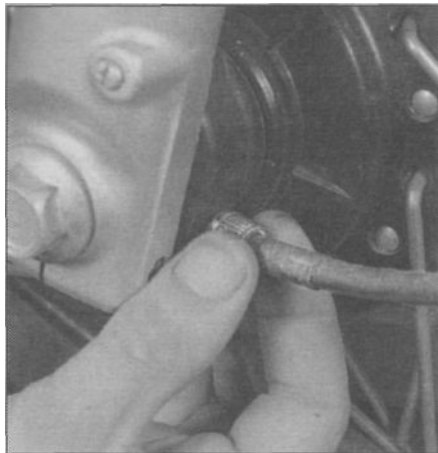
13.2 ... and from the drive unit on the left fork leg
