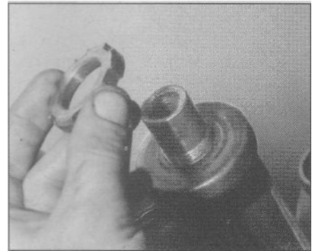
6.18c Install the ring nut and adjust the bearings
