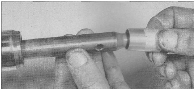
5.14 Fit the oil lock piece onto the exposed end of the damper rod
