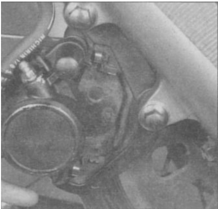
2.2b ... and pivot the caliper up to expose the pads
