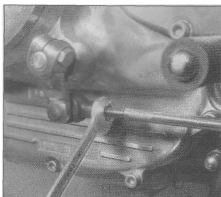
27.4 Loosen the locknuts and rotate the rod to change its length; on some models, the front nut has left-hand threads (loosens clockwise)
