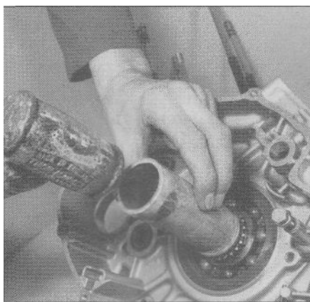
15.13c ... and drive the sprocket all the way on with a hammer and piece of pipe
