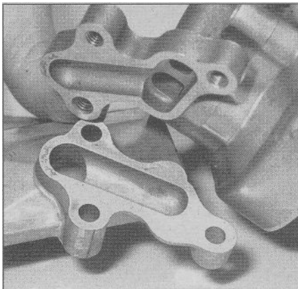
15.6b Remove three Phillips screws and detach the pick-up from the pump
