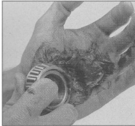
5.20 Work the grease completely into the rollers
