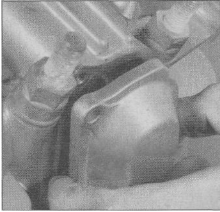
8.5 Unbolt the rocker arm covers and take them off, together with their O-rings
