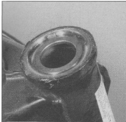
6.11d ... the race should look like this when installed
