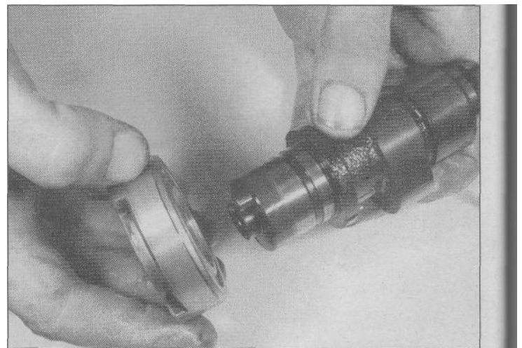
8.23b ... and take the bushing off the camshaft
