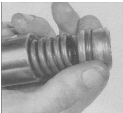
3.4b ... then remove the spring seat with its O-ring and the spring
