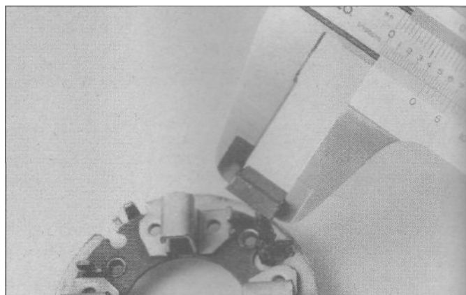
25.8 Measure the length of the brushes and compare the length of the shortest brush with the length listed in this Chapter's Specifications (four-brush starter shown; twp-brush model similar)
