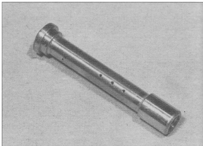
7.17c Check the needle jet for wear and clogged holes
