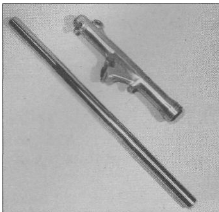
8.9a Inspect the inner and outer fork tubes; they must be replaced if worn or damaged
