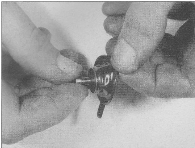
7.28 Check the coasting enricher solenoid diaphragms for cracks or brittleness
