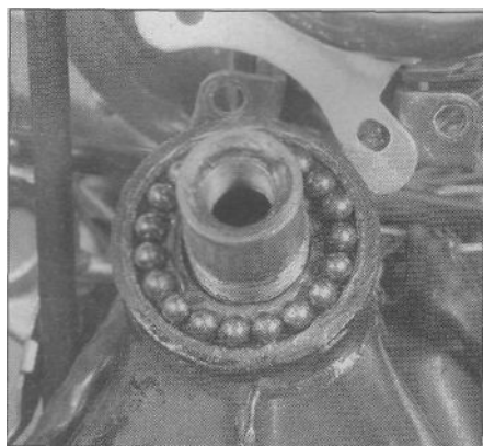
6.7d Remove the 19 steel balls
