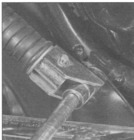
10.4 Unbolt the bracket at the right passenger footpeg
