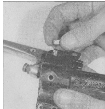
5.7a Remove the locknut from the lever pivot bolt...
