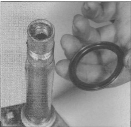
6.14a Install a new seal with its concave side down . .
