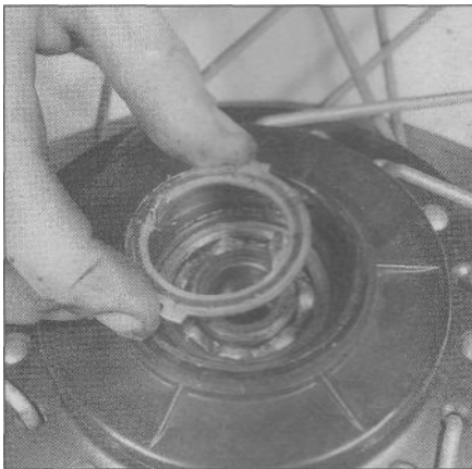
13.12a Install the speedometer clutch ...
