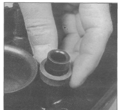
14.7b ... and the seals inside the filter housing; replace them if they're deteriorated or brittle
