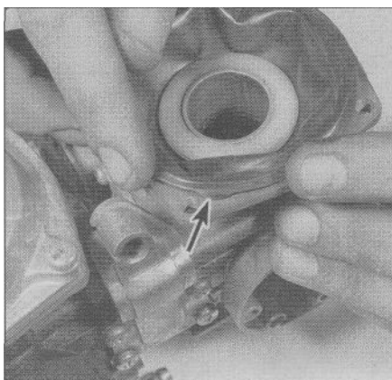
7.32b Align the protrusion in the diaphragm with the notch in the carburetor body (arrow)
