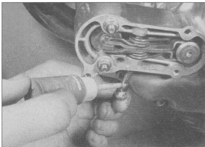
30.21 Apply non-permanent thread locking agent to the threads of the pivot bolt
