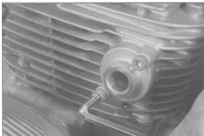
7.2a Remove the tensioner Allen bolts ,
