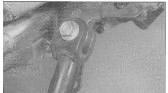
6.2 Remove the sidestand pivot nut and slide it off the post
