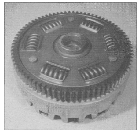
17.22 Check the driven gear teeth for wear or damage
