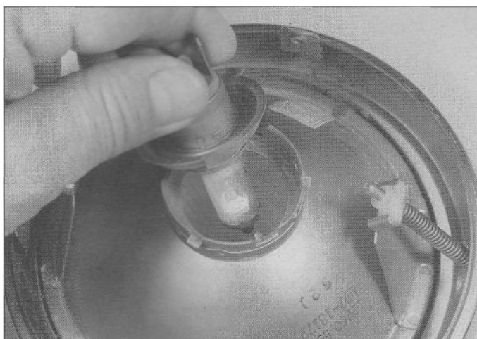
7.2b ... and lift the bulb out; don't touch the glass on the new bulb
