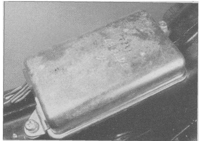
4.3 The igniter is mounted under the fuel tank on 1981 through 1983 models (shown) or forward of the rear fender on 1984 and later models
