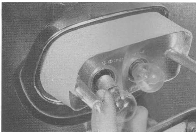
10.6 Press the bulbs into their sockets and turn counterclockwise (anti-clockwise) to remove
