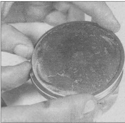
13.11a Install the middle ring with its identification mark up
