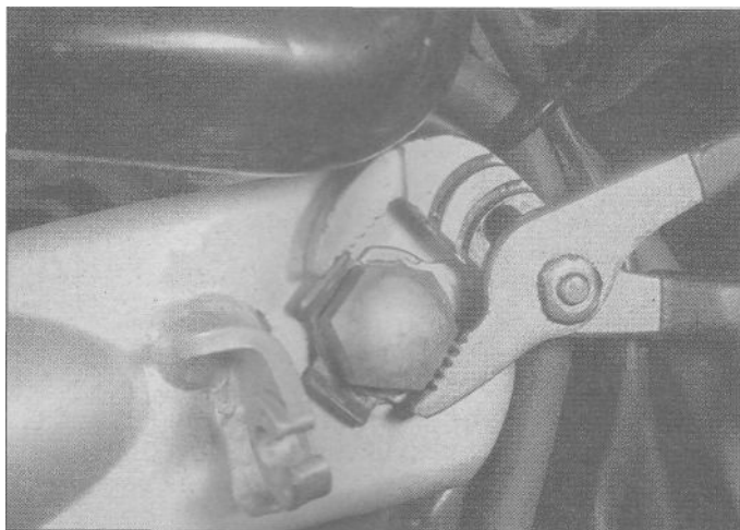
10.9 Bend the lockwasher tabs against the head of the pivot shaft
