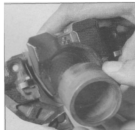
3.5b Remove the piston from the bore
