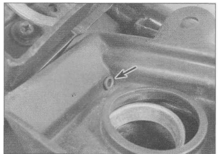
2.13 Work the drain fitting (arrow) free of the rubber cover and lift the cover out
