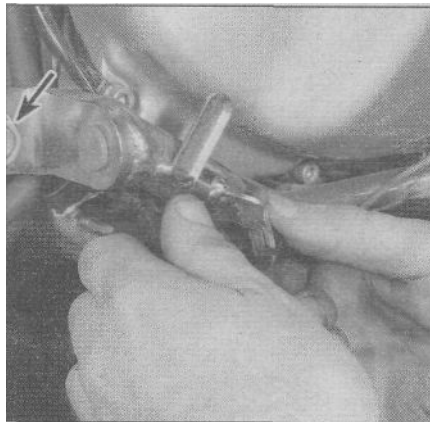
3.9b Follow the wiring harness from the brake light switch and disconnect the connector; remove the mounting nut (arrow)...
