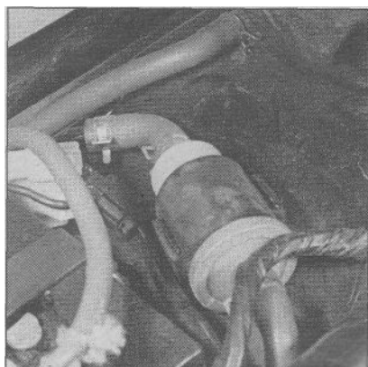
25.11 Loosen the clamp and disconnect the hose at each end of the filter, then remove it from its bracket
