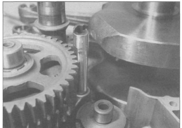
26.27b ... and align its flat with the teeth of the middle drive gear
