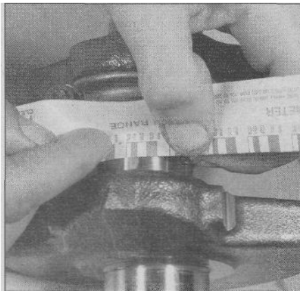
26.13 Place the Plastigage scale next to the flattened Plastigage to measure the bearing clearance
