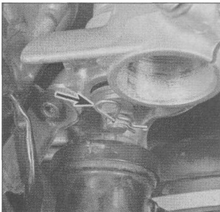
2.5 Pull out the clip (arrow) and remove the nut and washers to detach the bracket from the triple clamp
