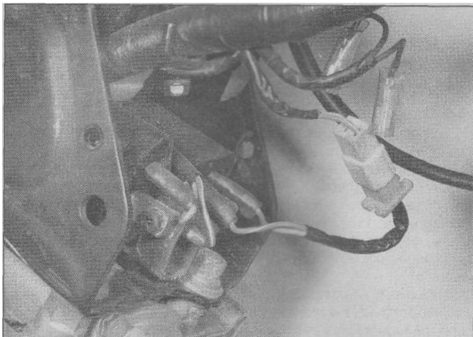
3.9 Disconnect the coil primary connectors (arrows)
