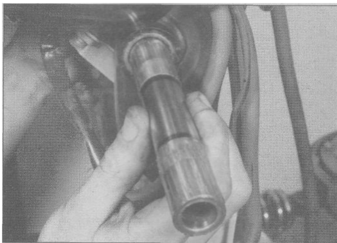
11.3 Pull out the bushing
