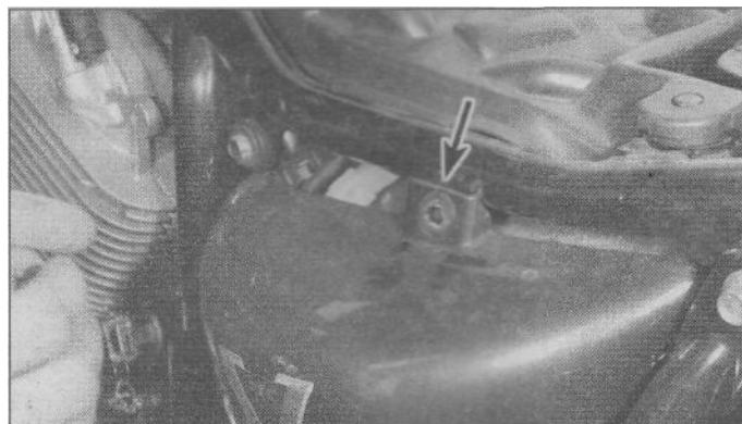
9.1 Remove the bolt from the mounting tab (arrow), then disengage the cover tabs from the slot and grommet
