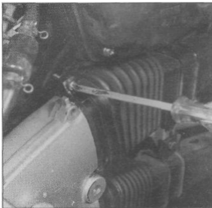
13.4 Loosen the screws on the chain case clamps
