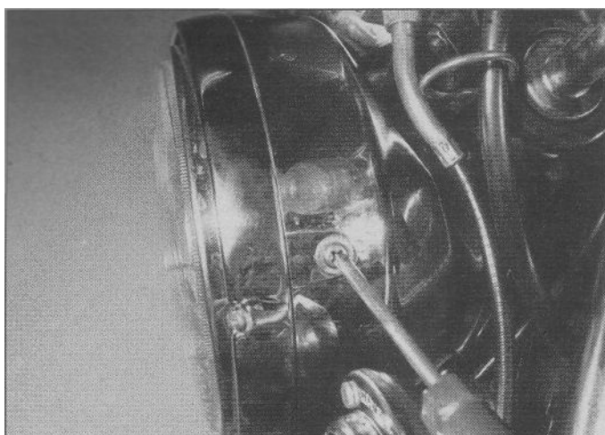
7.1a Remove the headlight cover screws .
