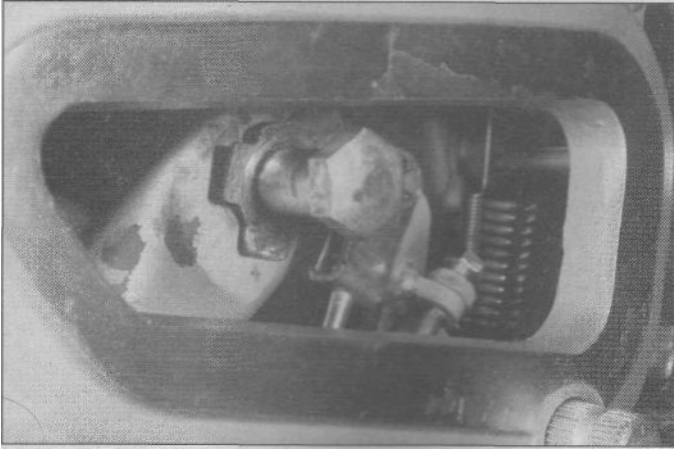
14.7b The pivot bolt head on 1981 through 1983 shaft drive models is secured by a lockwasher
