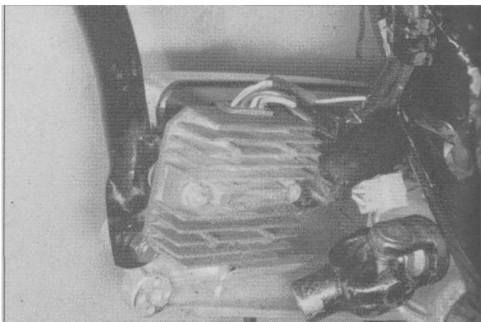
28.14 The voltage regulator/rectifier on 1981 through 1983 models is mounted on the rear subframe
