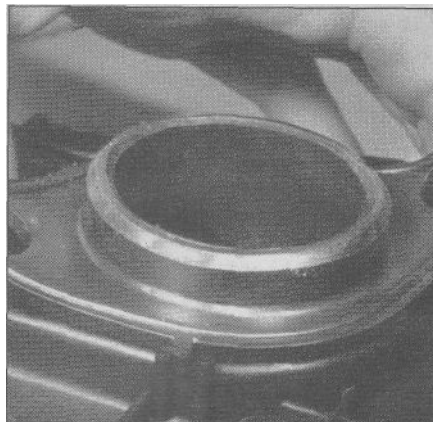
14.7a Check the seal between the filter housing and the frame ...
